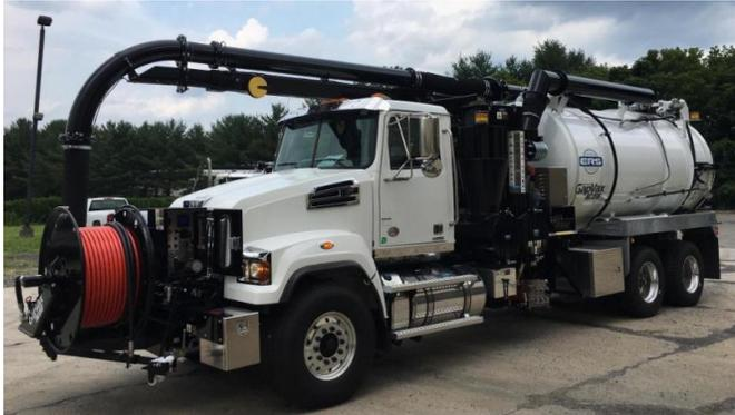
The GapVax MC Series Unit, Combination JetVac, is a wet only machine, equipped with a unitized water and debris tank and double sub-frame. With a wide variety of sizes available, this is an ideal candidate for any size municipality, water and sewer district, or contractor who is cleaning storm drains, catch basins and/or sewers.
