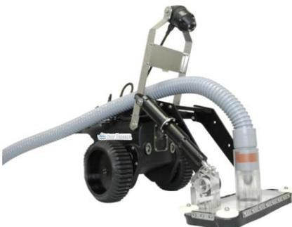
**DT640 Vacuum Crawler** - The DT640 Utility Crawler is the most versatile inspection vehicle of its kind. The sleek, three-wheel submersible comes with a magnetic option, creating the ideal vehicle for an array of underwater work. Compact for transportation and extremely portable, our Utility Crawlers have been designed to launch immediately for any location, and with the efficiency of internal batteries, they can provide up to 8 hours of work in a single 1.5 hour charge.
